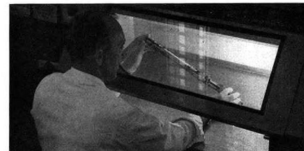
ELECTRONIC GUN is assembled under glass hood by technician wearing lint-free gloves.
