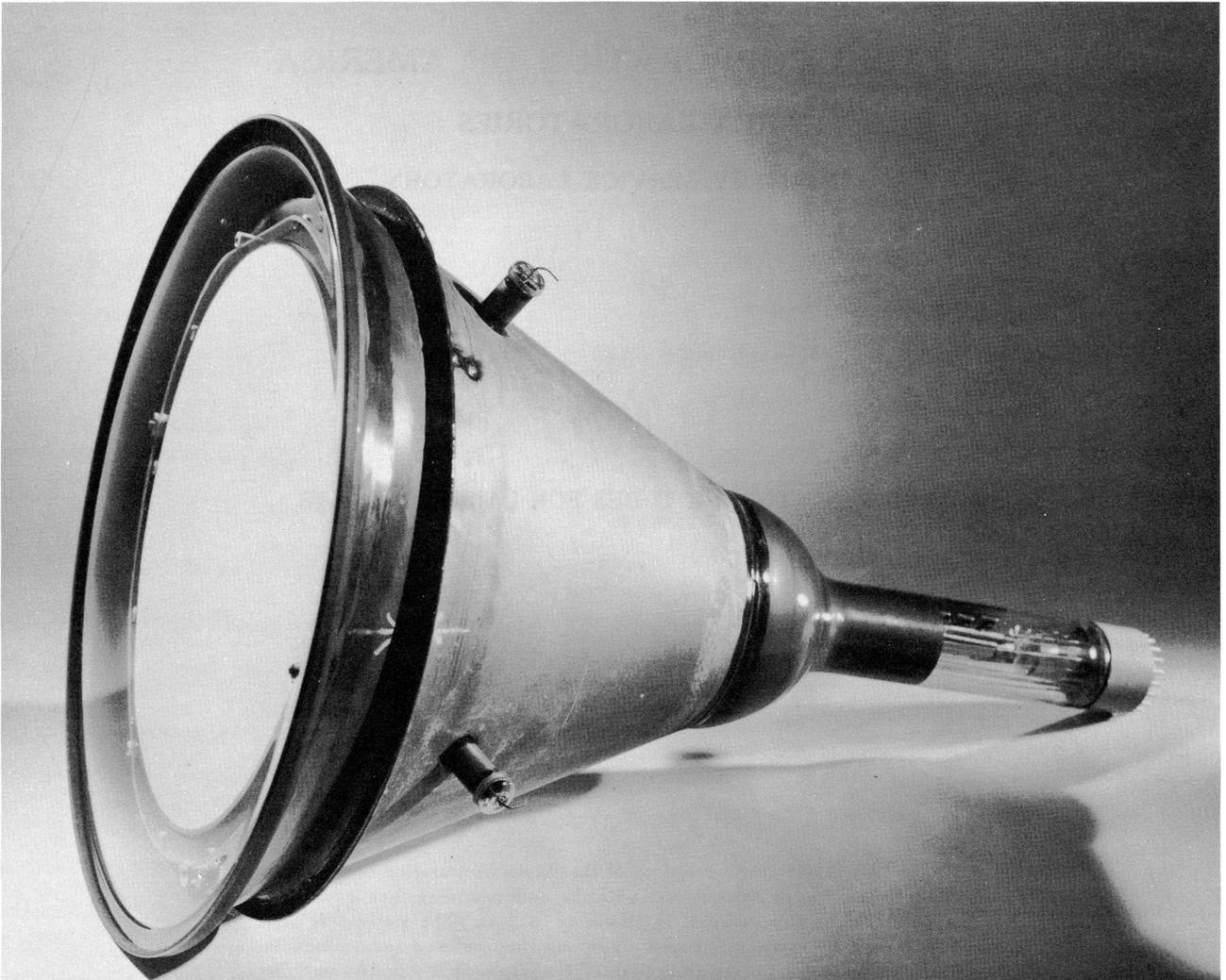
Fig. 1 – Direct-view storage tube with 10-inch diameter target.
