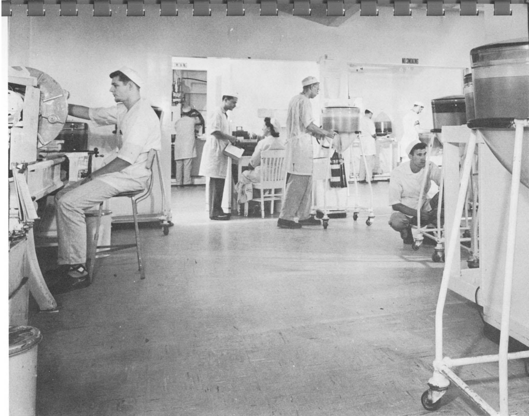
MAIN TUBE MANUFACTURING AREA. In the far right, technicians are applying the phosphor screen to the tube; in the left foreground, a technician is applying the helical accelerator anode to the inside of the tube. Hospital-like environmental conditions are maintained to insure perfection in finished tube products.
