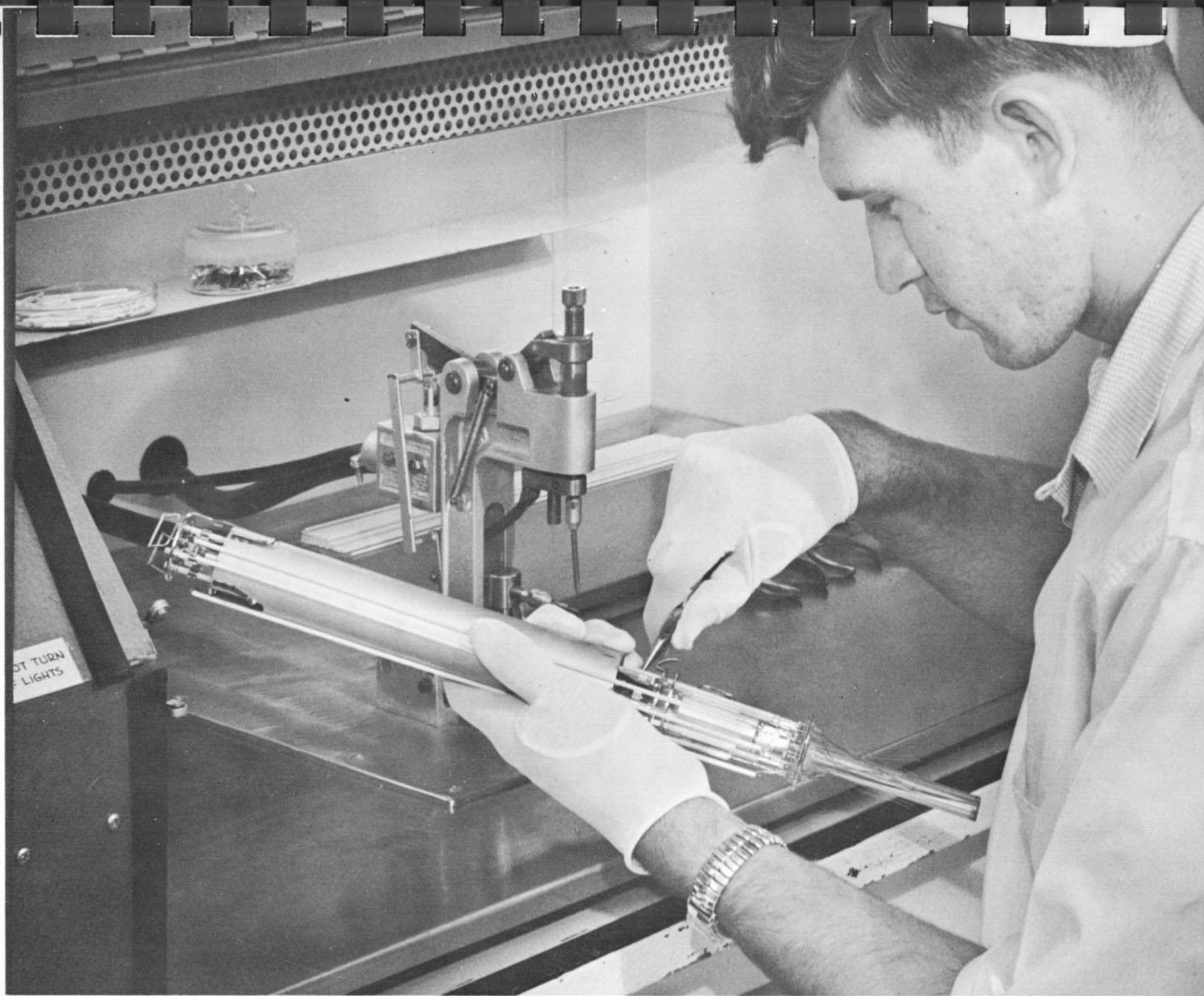
ASSEMBLY OF ELECTRON GUNS FOR CHARACTER SHAPED BEAM TUBE. Extensive care has been taken to protect the delicate components of the electron gun from contamination during its close-tolerance assembly.
