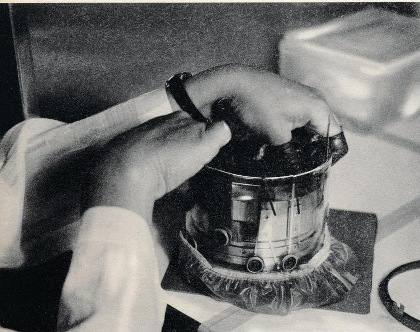
Insertion of target-mesh assembly in the glass cylinder
