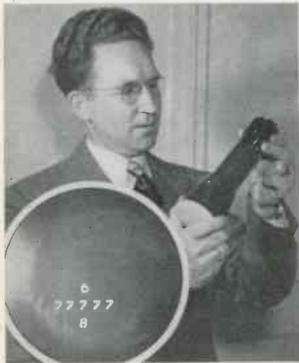
J. T. McNaney, inventor of the Charactron, is shown examining one of the experimental tubes. The tube is the chief component of Electrontype, a new method of high speed communication (see TELE-TECH, March, '49, p. 47). Inset is closeup view of Charactron used for numerical displays. McNaney conducted experiments at the Consolidated Vultee Aircraft Corp., San Diego, Calif.
