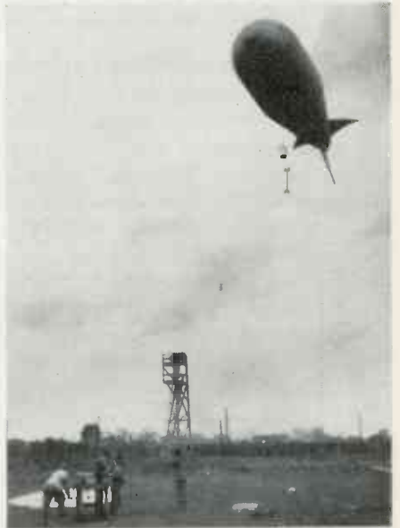
A helium-filled balloon carrying a pulse transmitter and antenna is raised by RCA engineers who are studying TV transmission characteristics of site in the Philadelphia area. Receiving unit is mounted in a truck and is powered by a motor generator
