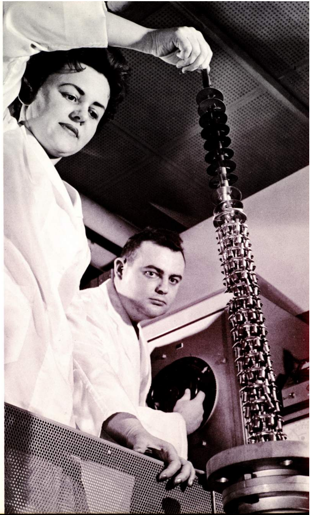
Coating uniformity of new "Sarong" cathode, right, compared with conventional type
